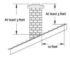
Chimneys shorter than 14 feet may not provide adequate draft. This could result is smoke spilling into the room from the stove when loading the stove, or when the door is open. In addition, inadequate draft can cause back puffing, which is a build up of gases inside the firebox.
